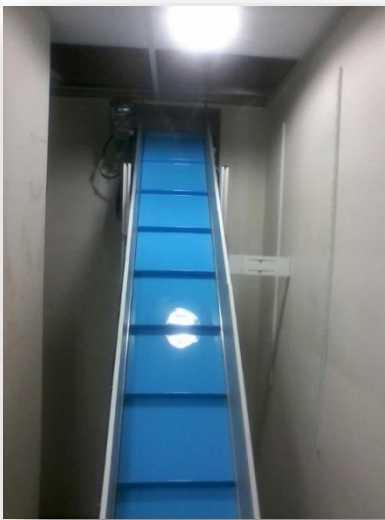
Inclined conveyor belt
